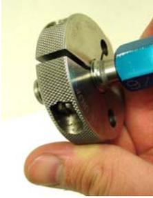
Evaluating the flank angles on the Truncated section of the Setting plug.
